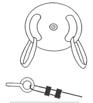
Note: 2 cable ties are to be used \*Try to put the second tie covering the dead end of the wire for safety
