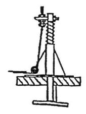
For any type of brake make sure the brake lining (a piece of old tire, for instance) is very well attached to the brake shoe.
