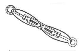
All turnbuckles must be wired or securely fastened in the event that the turnbuckle loosens up
