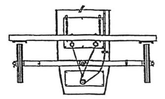
The drop arm brake is a popular design among true racers because it can be designed to remain flush with the body until the finishing line, and thus minimize wind drag (see examples). It can be constructed relatively easily by you.
